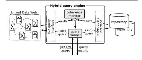
Figure 6.2: Architecture of a hybrid query engine.
