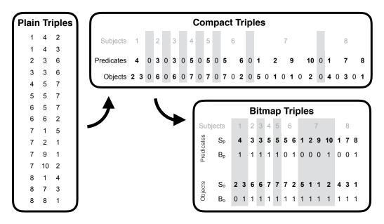
Figure 13: Three encodings for triples in HDT.
