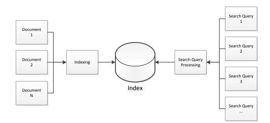
Figure 1: Core Architecture of a Search Engine
